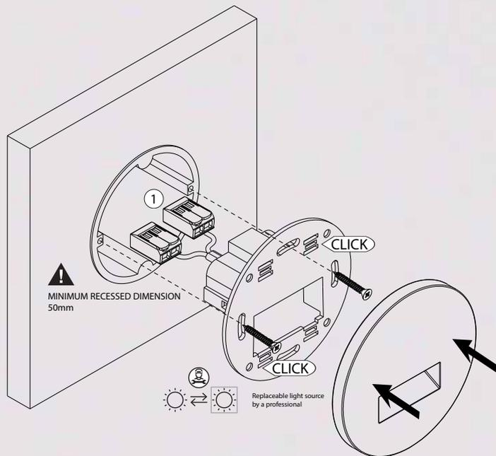
**i** Fits on standard round electrical junction box with screws (hole dia 68mm)
